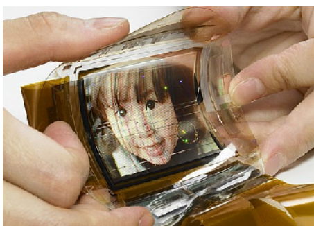
Sony unveiled what it is calling the world's first flexible, full-color OLED display built on organic thin-film transistor (TFT) technology
